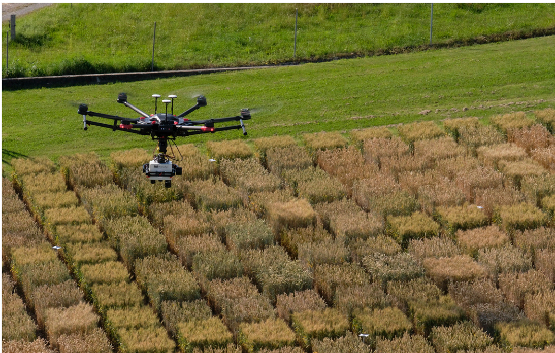
Researchers at ETH Zürich use standard color images and thermal images collected by drone to determine how plots of wheat with different genotypes vary in grain ripeness. Image credit: Norbert Kirchgessner (ETH Zürich, Zürich, Switzerland).
